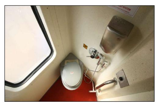
Shower Cubicles with Hot & Cold Running Water is available on board. Lavatories are equipped with Bio Toilets with Vacuum evacuation.
